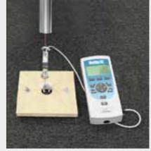
Testing of fixing element strength
